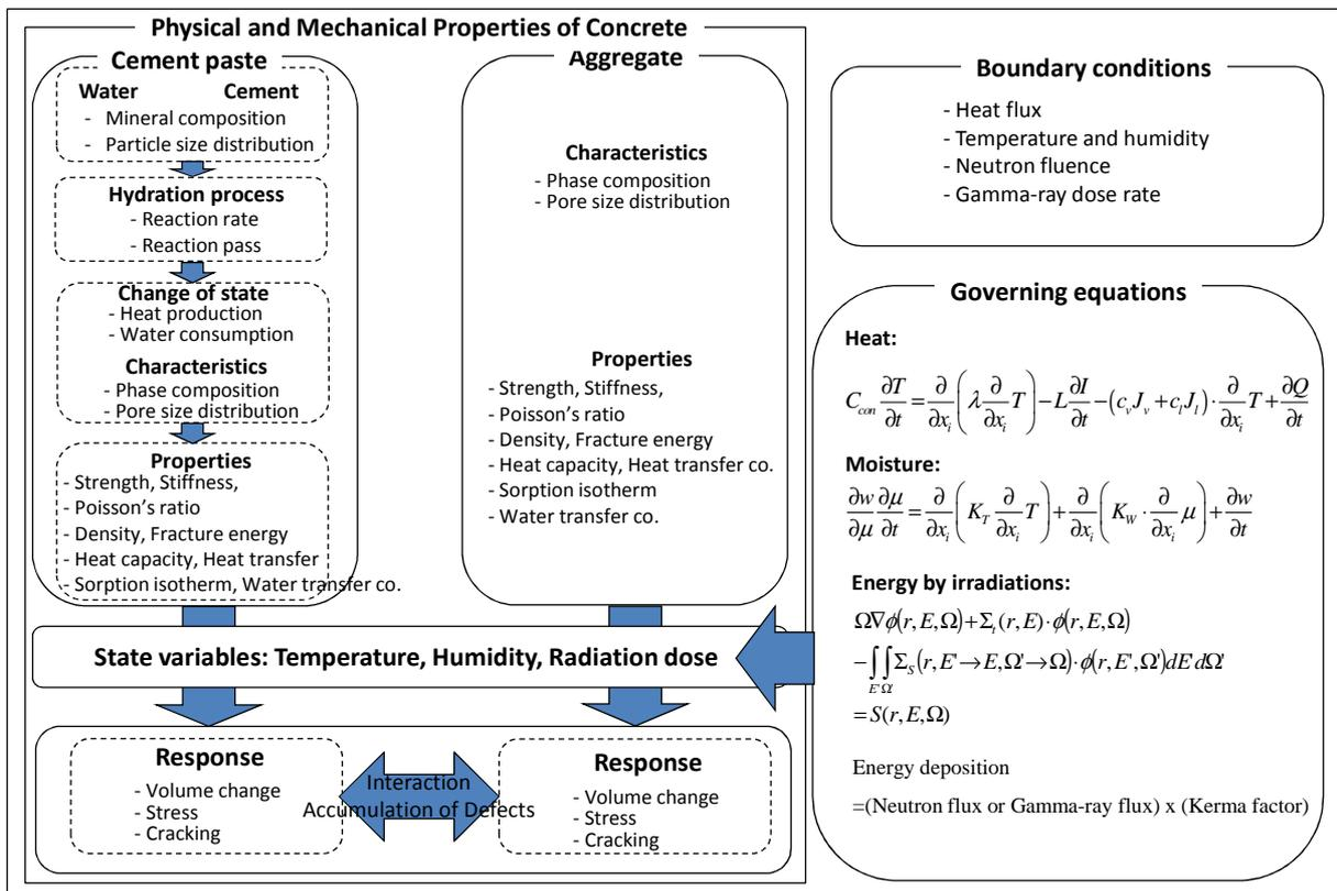
FIG.4 Diagram of numerical simulation for concrete deterioration under irradiated conditions.
