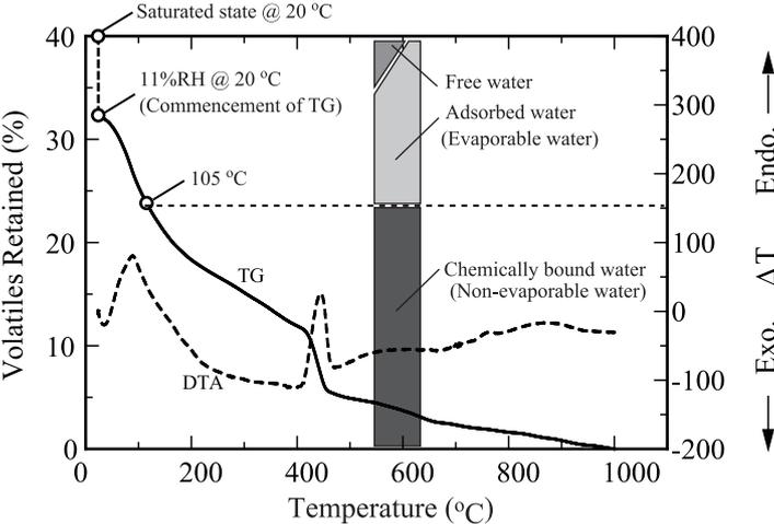
FIG.2 Types of water in cement paste with TG-DTA data of ordinary Portland cement paste.
