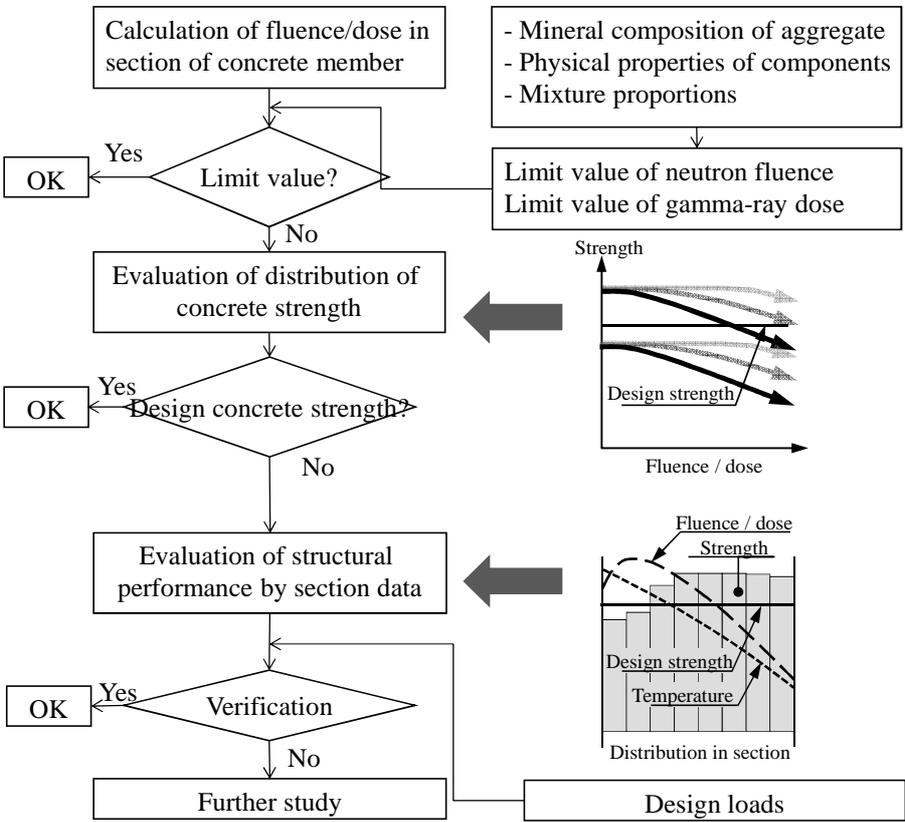
FIG.5 Assessment flow chart for soundness of concrete member exposed to radiation.
