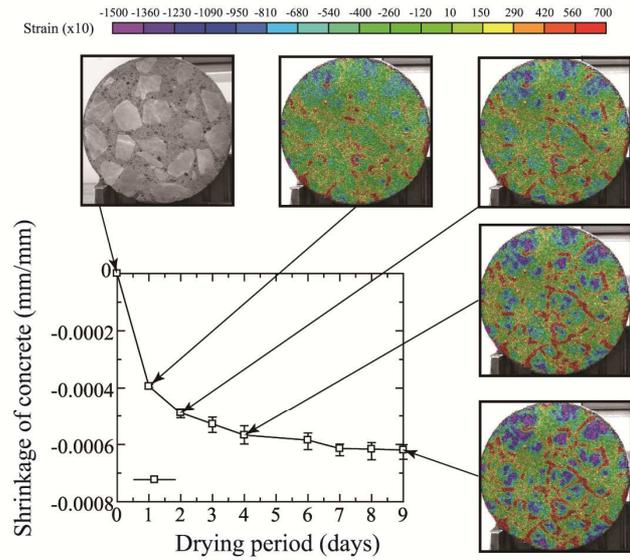
(a) Shrinkage strain of cement paste and aggregate
