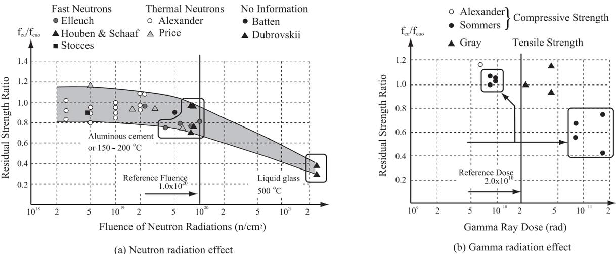
FIG.1 Residual strength ratio of concrete exposed to neutron radiation (a) and gamma radiation (b). (after [1], some notes are added together.)
